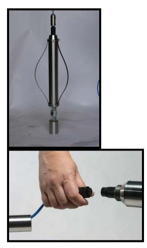
Thread the cable head through the centralizer and the cable head cover sleeve and connect the camera.
