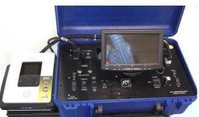
The R-cam1000 Color Video Water Well Inspection System is equipped with two cameras in a single housing, each with a wide-angle lens, for viewing down hole and side view images in water wells or boreholes. Low light level CCD sensors allow the cameras to detect images with minimal lighting power, as low as 1 LUX.
