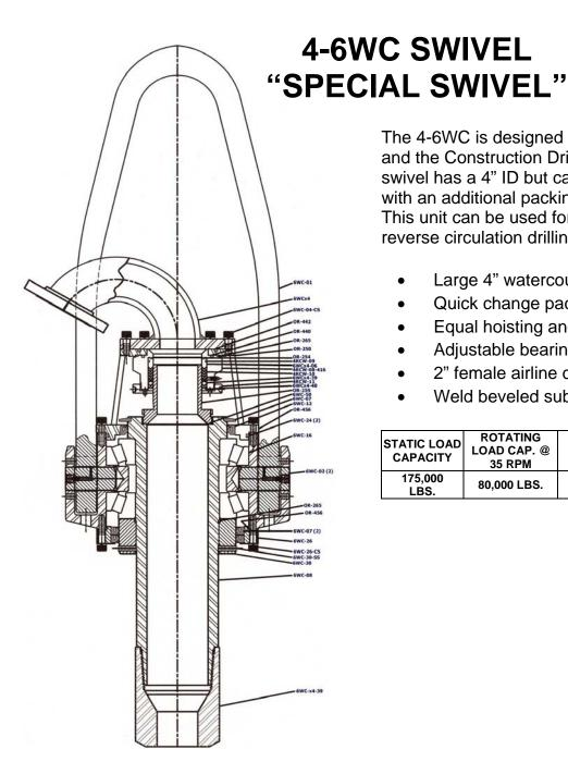
The 4-6WC is designed for the Water Well Irrigation, and the Construction Drilling Market. This compact swivel has a 4" ID but can be converted to a 6" ID with an additional packing capsule and gooseneck. This unit can be used for both conventional and reverse circulation drilling.
