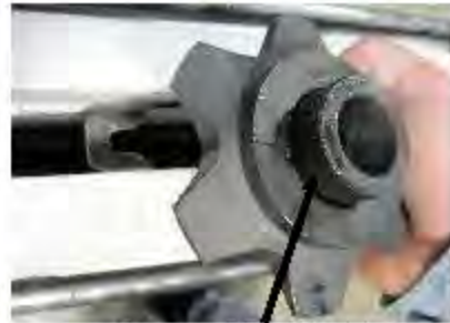
Grease OD of Bushing
